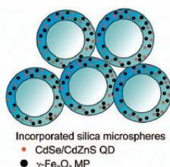
**Figure 9.** Magnetic and fluorescent silica microspheres fabricated by incorporating maghemite ( $\gamma\text{-Fe}_2\text{O}_3$ ) nanoparticles and CdSe / CdZnS core / shell quantum dots into silica shell around preformed silica microspheres of sizes  $\sim 500$  nm [24].
