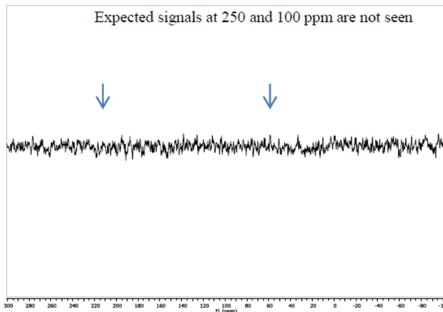
**Figure 2.**  $^{15}\text{N}$  NMR spectra of 100 mM sodium azide.
