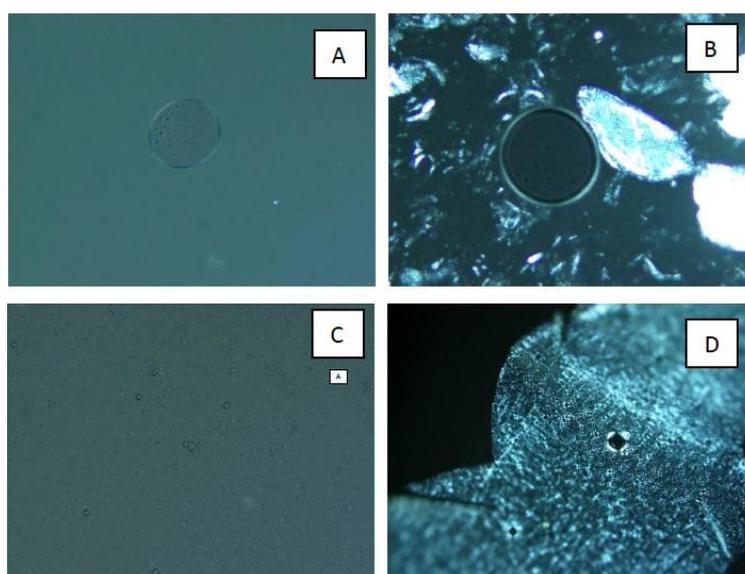
**Figure 8.** Micrograph of Curcumin in A) the simple emulsion (20 ×). B) the double emulsion by 5 wt. % chitosan solution (20 ×). C) the coacervated microcapsule (prior to freeze-drying) (10 ×). D) freeze-dried coacervated microcapsules (10 ×).
