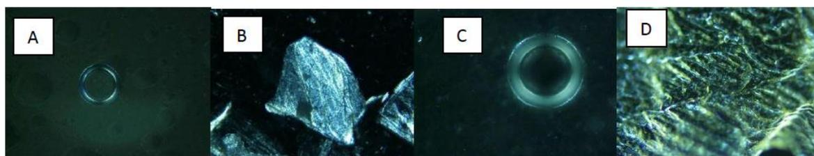
**Figure 4.** Blank micrograph of A) the simple emulsion (20 ×). B) the double emulsion by 5 wt. % chitosan solution (40 ×). C) the coacervated microcapsule (prior to freeze-drying) (40 ×). D) freeze-dried coacervated microcapsules (10 ×).
