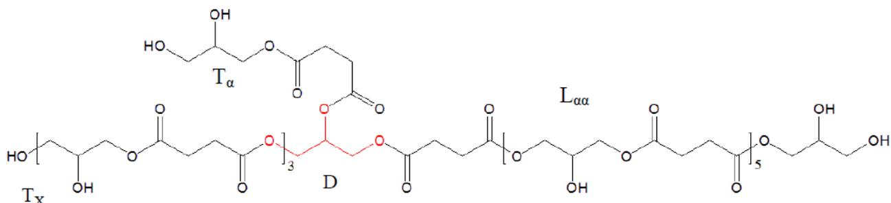
**Figure 1.** Chemical structure of PGSs, with terminal units ( $T_x$ ,  $T_\alpha$ ,  $T_\beta$ ), linear units ( $L_{\alpha\alpha}$ ,  $L_{\alpha\beta}$ ) and the dendritic unit (D).  $R = \text{CH}_2\text{-COOH}$  when  $T_x$  is a succinyl,  $R = \text{H}$  when  $T_x$  is non-grafted and  $R = (\text{CH}_2)_n\text{-CH}_3$  when  $T_x$  is a acyl group of fatty acid.
