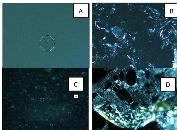
**Figure 6.** Micrograph of ascorbic acid in A) the simple emulsion (20 ×). B) the double emulsion by 5 wt. % chitosan solution (20 ×). C) the coacervated microcapsule (prior to freeze-drying) (10 ×). D) freeze-dried coacervated microcapsules (10 ×).
