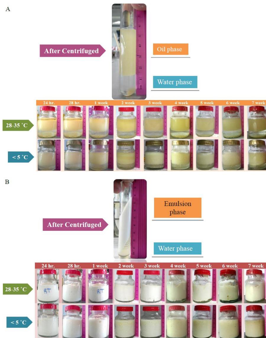
**Figure 2.** A) Water: RBO (with PG<sub>1.5</sub>SF<sub>R0.05</sub> 2.5 wt. %) in a ratio of 50 : 50; B) Water (with gum Arabic 5 wt. %): RBO (with PG<sub>1.5</sub>SF<sub>R0.05</sub> 5 wt. %) in a ratio of 50 : 50.
