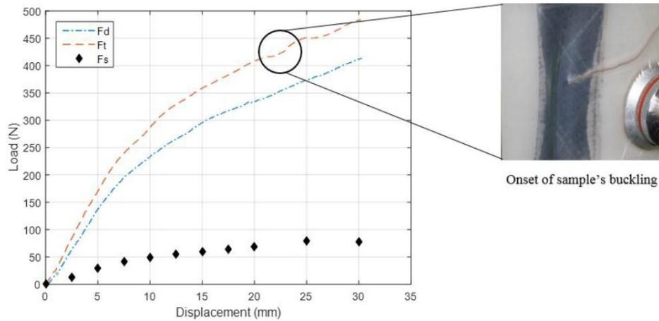
**Figure 3.** Load-displacement response to the bias extension test under 100 kPa compaction at 50 °C.  $F_s$  indicates the load needed to extend the prepreg sample;  $F_t$  is the total measured load of the bias extension setup with the prepreg sample;  $F_d$  is the load required to extend the bias extension setup without the prepreg sample.
