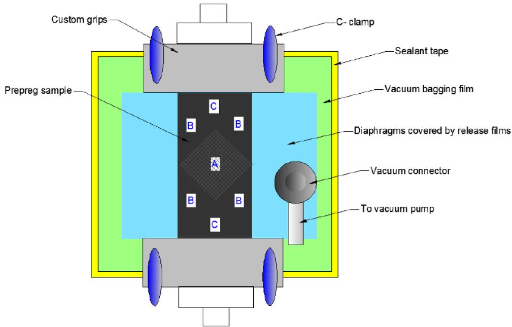
**Figure 2.** Bias extension setup under diaphragm forming compaction.
