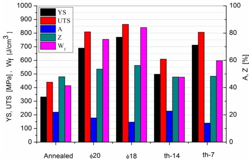
**Figure 5.** Mechanical properties of industrially rolled titanium samples. YS: yield strength, UTS: ultimate tensile strength, A: elongation to failure, Z: reduction in area, W<sub>f</sub>: strain energy density to fracture. The experimental error of the values is about 8 %. φ20: sample from product 1, φ18: sample from product 2, th-14: sample from product 3, th-7: sample from product 4 (see **Table 4**).
