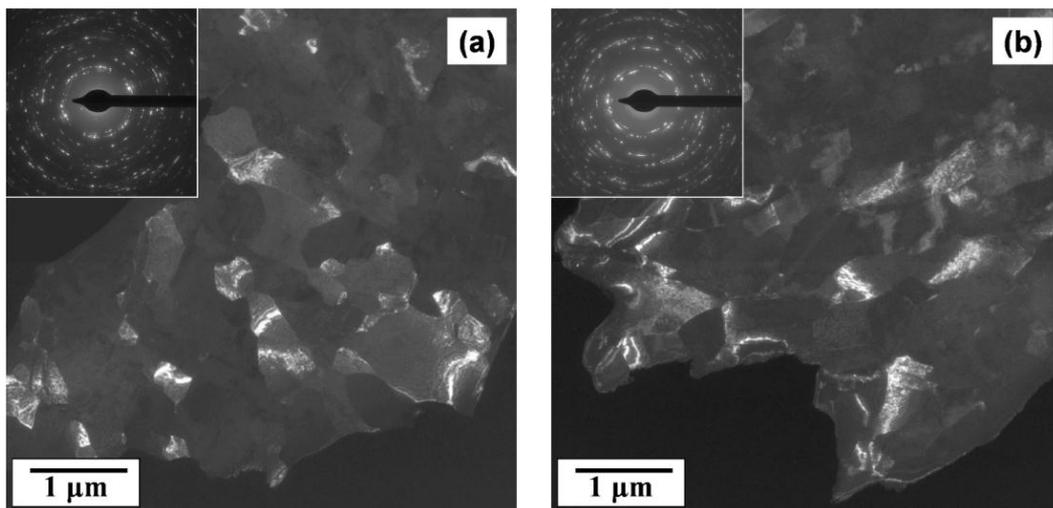
**Figure 10.** Dark field TEM images of the grain structure in industrially rolled Grade 2 titanium. (a) cross- and (b) longitudinal sections. The rolling direction is vertical in figure (b). The insets show the corresponding diffraction patterns.
