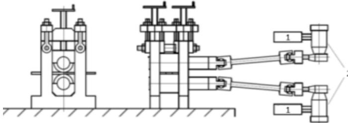
**Figure 1.** The sketch of the experimental roll stand for caliber rolling. 1 – speed control, 2 – twin motor drive.
