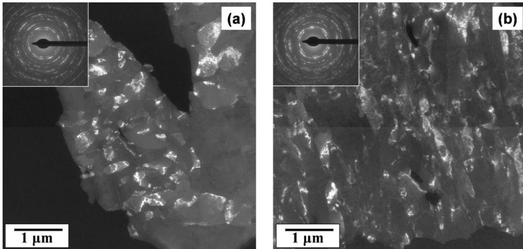
**Figure 9.** Dark field TEM images of the grain structure in laboratory rolled Grade 2 titanium. (a) cross- and (b) longitudinal sections. The rolling direction is vertical in figure (b). The insets show the corresponding diffraction patterns
