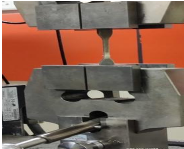
Figure 2: Full carbon composite laminate under tensile loading prior to failure
