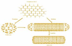
Figure 1: Single-walled carbon nanotubes closed at both ends
