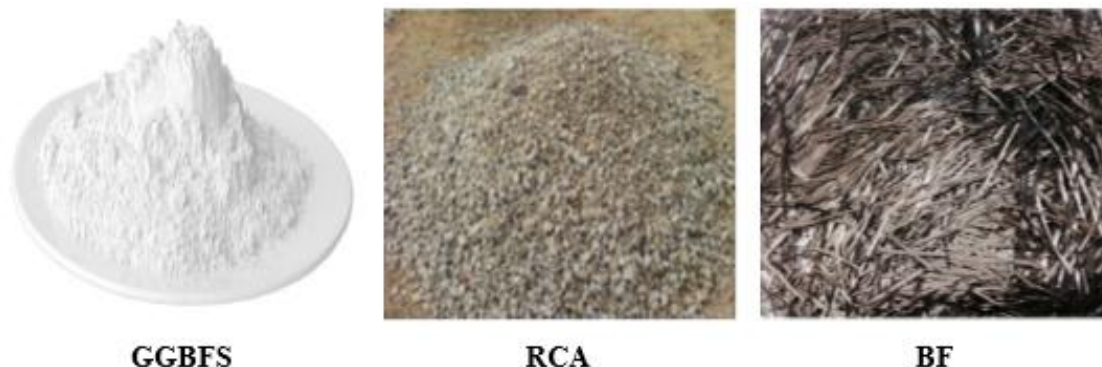
Figure 1 Main Ingredients of BFRC.
