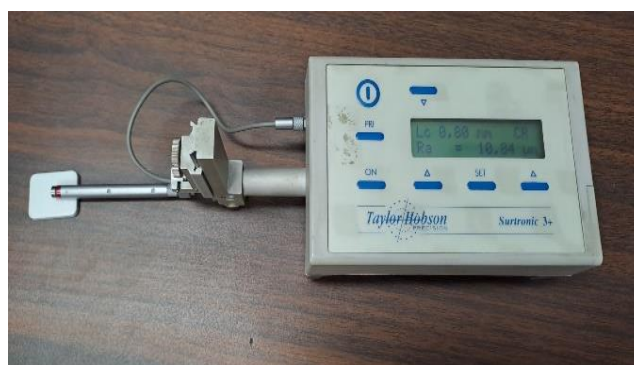
Fig 5. Taylor Hobson surface roughness tester with printed sample parts
