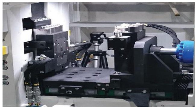
Fig.6 Linear FSW and specimen location. [49]
