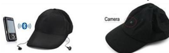
Fig. 9. Camera module embedded in a hat to take the input wirelessly
