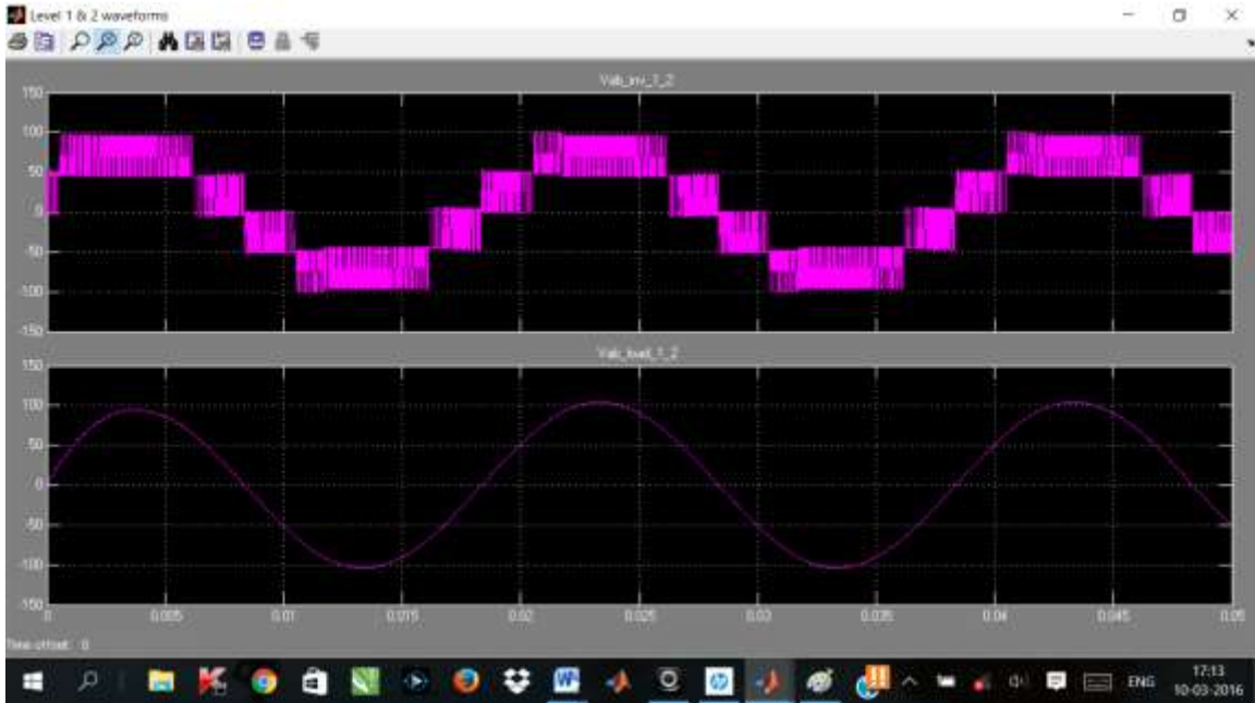
Fig. 7 : The o/p waveforms of the combined levels 1 and 2, including inverter output and load output, demonstrate a smooth output supply after the incorporation of the filter, resulting in the removal of all harmonics up to the 8th order.
