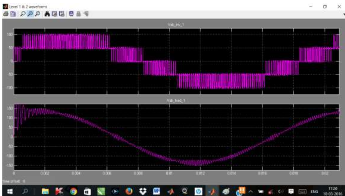
Fig. 6 : The waveforms of the combined levels 1 and 2 for the inverter output and load output are displayed, show harmonics content along with un-distorted supply's waveform, which have been zoom in.
