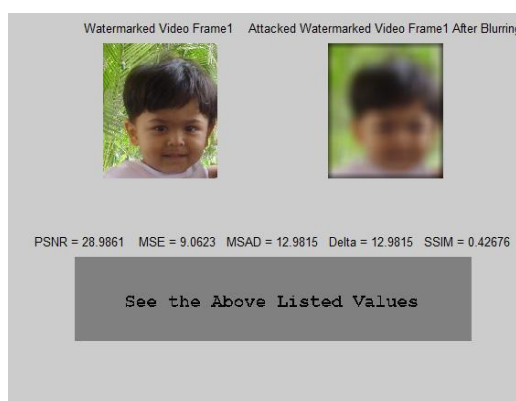
Fig. 12 Comparison of two frames on the basis of PSNR, MSE, MSAD, Delta and SSIM for Blurring Attack
