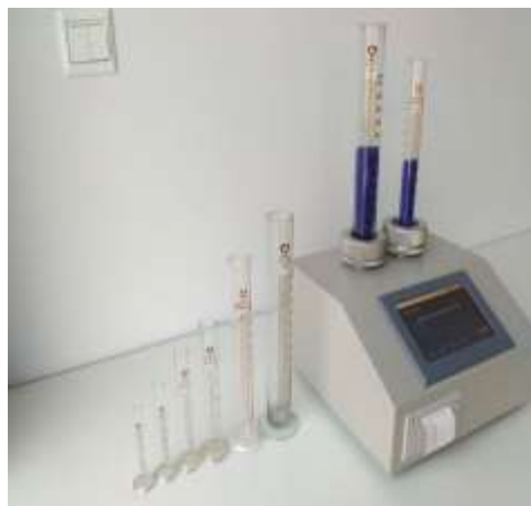
Figure 11: Determination of Bulk and Tap Density and Compressibility Index.
