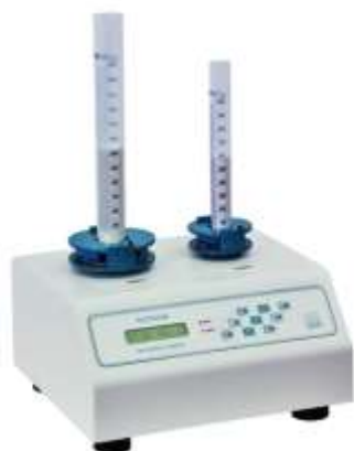
Figure 11: Determination of Bulk and Tap Density and Compressibility Index.
