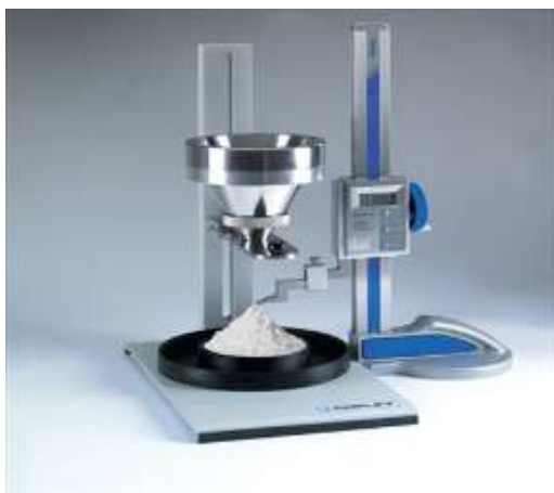
Figure 10: Determination of Angle of Repose and Flow Rate.
