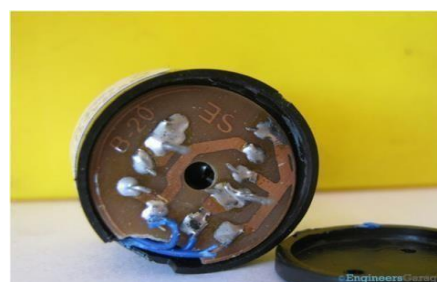
Fig. 2: Image Showing PCB and Electronic Components of Piezo Buzzer
