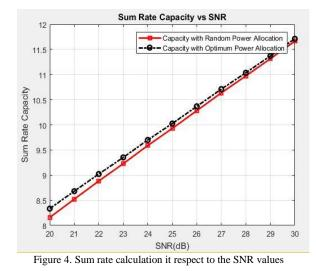
Figure 4 indicates the sum rate improvement when the SNR values increase. Thus using a relay at the secondary network improves the system performance by using optimal power allocation at the secondary network which improves the system performance ant throughput.
