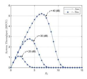
Figure 5: System throughput versus noise variance 20,30 and 40dB.
