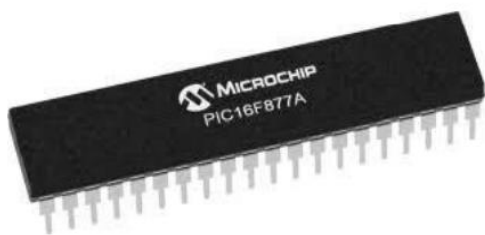
Fig-4: PIC Controller
