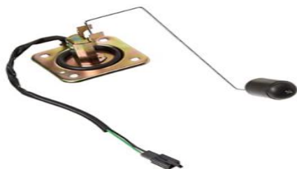
Fig-3: Fuel sensor
