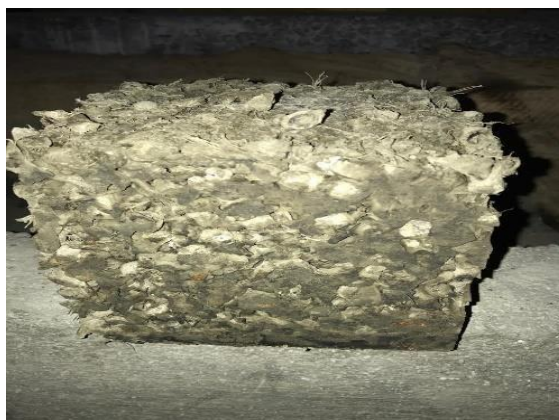
Fig.10: Non-treated OPS Concrete cube 150*150*150 mm
