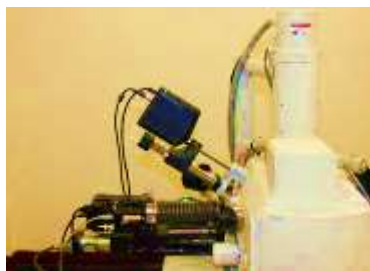
Figure 1 Layout of EDAX with TEM for Bruker X Flash 630 EDS Detector
