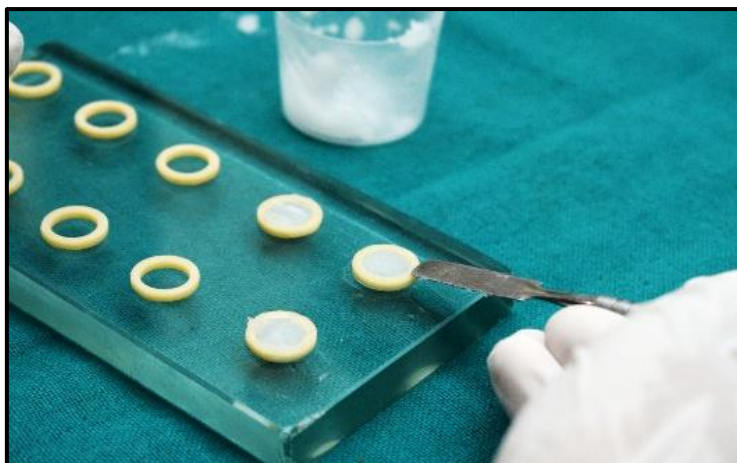
Figure 1: Fabrication of soft liner discs of 10mm x 2mm dimension
