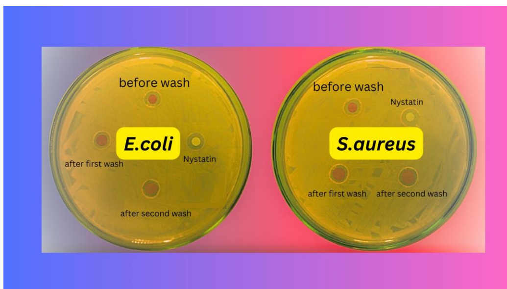
Fig. 1 Antibacterial activity of Nystatin treated organic cotton fabric against (A) Escherichia coli , and (B) Staphylococcus aureus .
