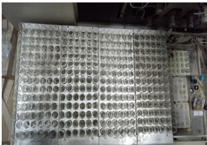
Figure 2. Collection of pure eluents in the test tubes
