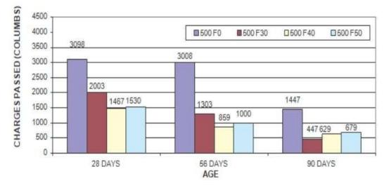
*RCPT Results of 500 Mix* Graphs & Charts based on w/c ratio & Compressive Strength of concrete
