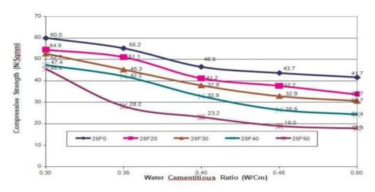
Compressive strength vs w/c ratio at 28 days
