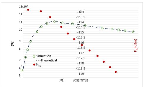
Figure 09. PU performance with a fixed SU value Pd = 0.25 and a range of SU (Pc, PSU) operating pairs on the 2nd-order polynomial boundary
