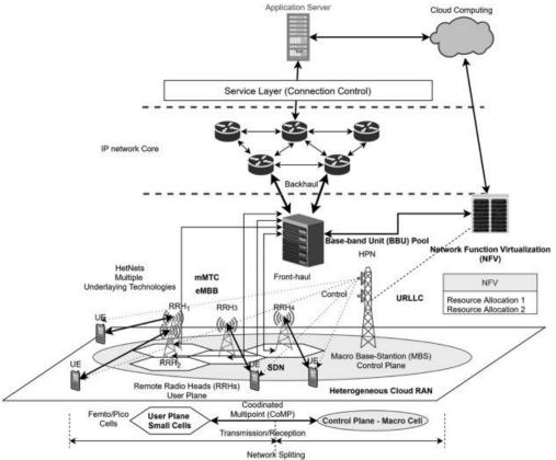
**Fig.3:** high-data rate/enhanced Mobile Broad-band (eMBB), ultrareliable low latency communication (URLLC), and massive Machine-Type Communication (mMTC)
