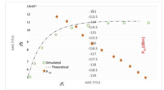
**Figure 07.** PU performance with a fixed SU value PY = .9 and a range of SU (Pc, PSU ) operating pairs on the 4th-order polynomial boundary.
