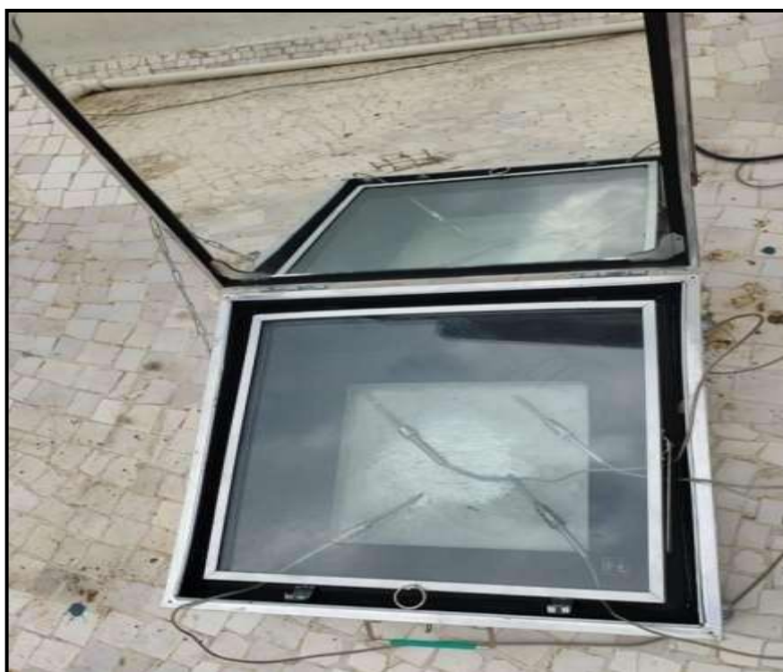
Figure 3: Experimentally Setup of Solar Still
