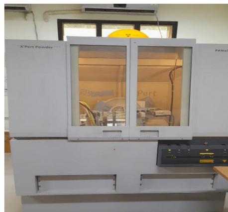
**Figure 4: Schematic Diagram of X-ray Diffractometer and its photograph**
