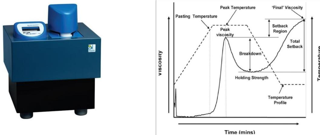
Figure 5: Rapid Visco Analyzer Experimental Setup and RVA Profile
