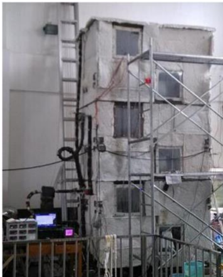
Fig. 7 Experimental setup of triple effect multi-effect HDH desalination system. (Gang et al. 2016)
