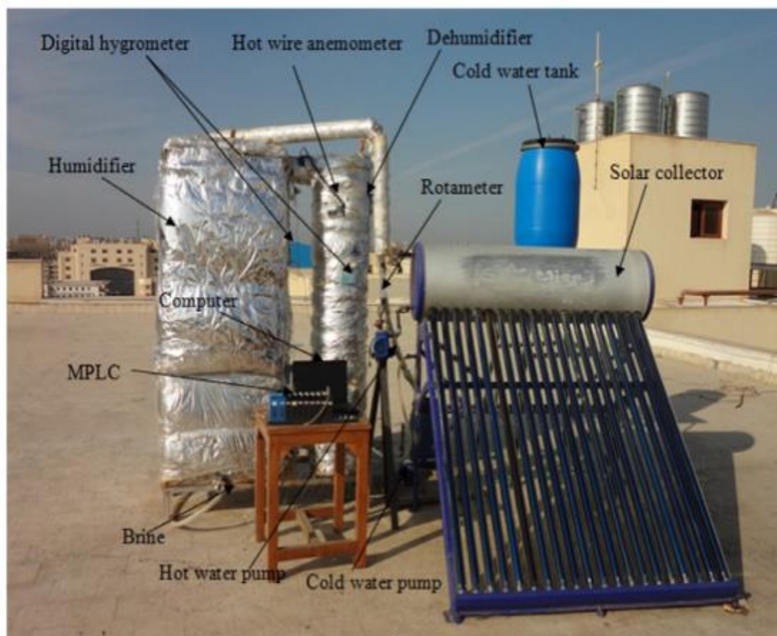
Fig. 5 Experimental setup of HDH desalination system with use of ETC (Hamed et al. 2015)
