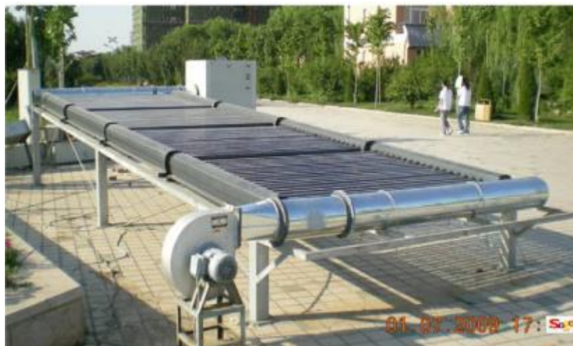
Fig. 4 experimental setup of pilot HDH desalination system with new design SAH and ETC ( Li et al. 2014)
