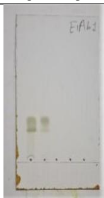
Figure 1: TLC estimation of all collected fractions of CSE (M) after column chromatography & Std Sterol
