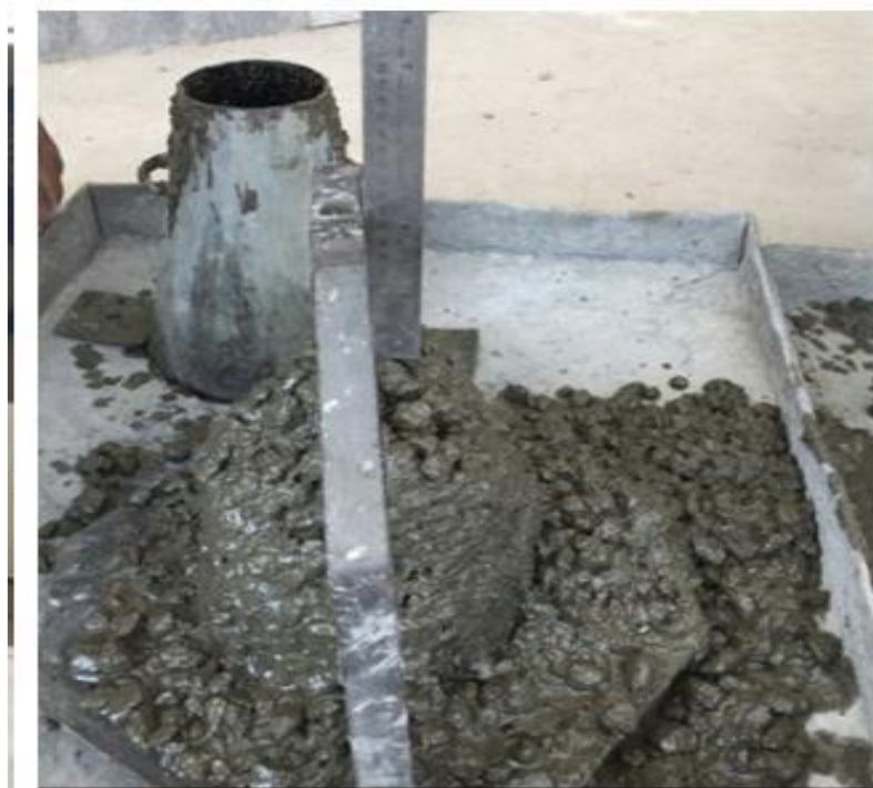
Figure 4: Slump Cone Test
