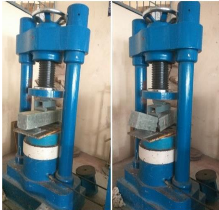
Figure 2: Flexural strength test
