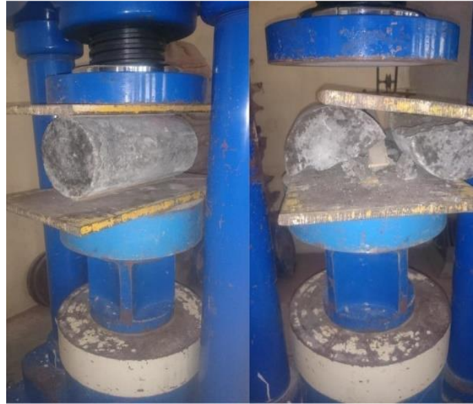
Figure 1: Split Tensile Test
