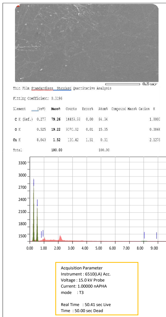
Figure 5. SEM-EDS image of CS(4%)-PVA-PPO- Cu 2+ membrane
