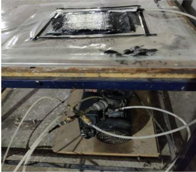
Figure 2. Vacuum infusion process
