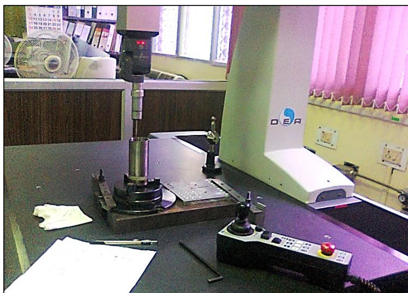
Figure 5. Form measurement using DEA 070705 CMM
