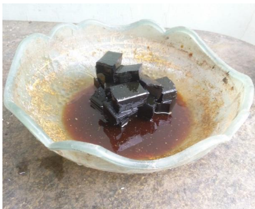
Fig.3 Mixing of Rubber Shreds with Resin Shreds (with resin)
