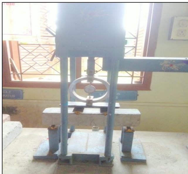
Fig.9 Test Set-up for Prism Specimen
