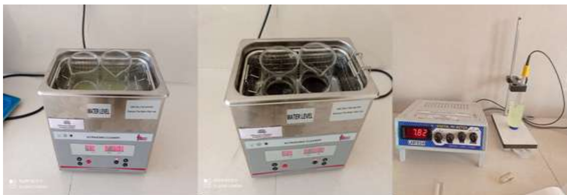
Figure 2.2 Photographs of Ultrasonication & PH measurement of Diesel+CuO+Gr, Diesel+Gr+Al 2 O 3 , and Diesel+Al 2 O 3 +CuO hybrid nano-diesel
