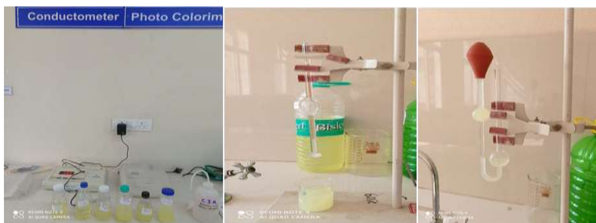
Figure 2.3 Measurement of thermal conductivity, surface tension & viscosity of Diesel+CuO+Gr, Diesel+Gr+Al 2 O 3 , and Diesel+Al 2 O 3 +CuO hybrid nano-diesel
