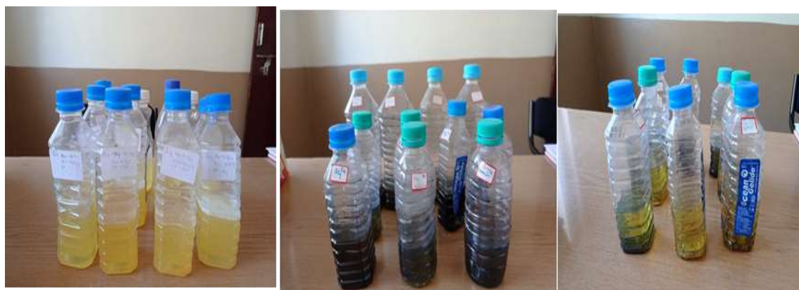
Figure 2.1 Samples of Diesel+CuO+Gr, Diesel+Gr+Al 2 O 3 , and Diesel+Al 2 O 3 +CuO hybrid nano-diesel
