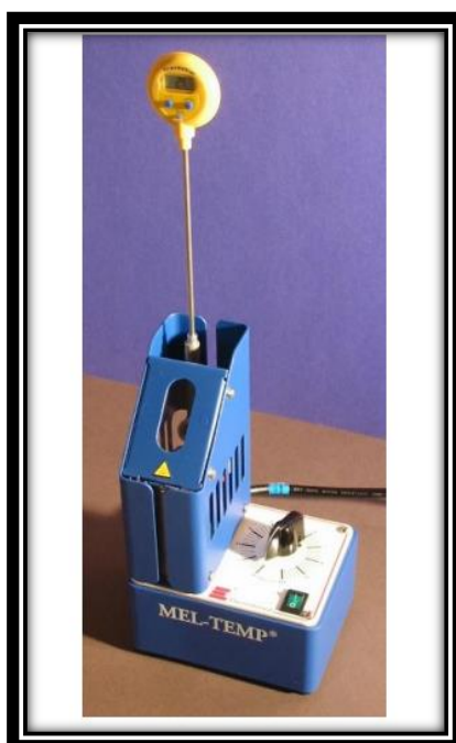
Figure 1 Melting-Temp apparatus equipped with a digital thermometer
