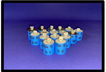
After that the fracture resistance of the specimens was measured with a Universal Testing Machine (P.S.I. Sales Pvt. Ltd., New Delhi) above the cingulum at a crosshead speed of 5mm/min at a 130 degree angle with the long axis of the root. The forces necessary to fracture each tooth were recorded in Newtons.
