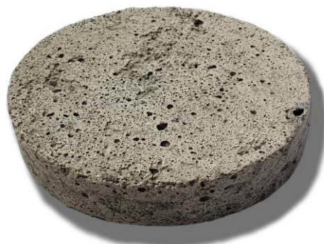
Figure 6. Geopolymer binder based on waste slag, natural sand and phosphoric acid (sample No. 8)
