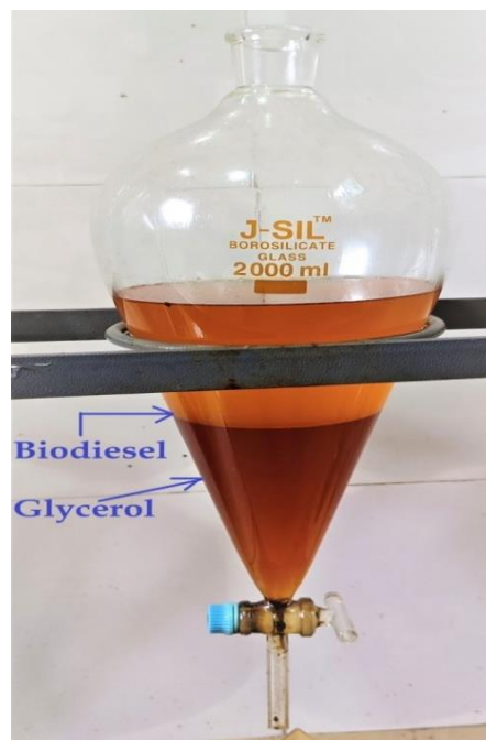
Figure 3: Biodiesel and glycerol separation
