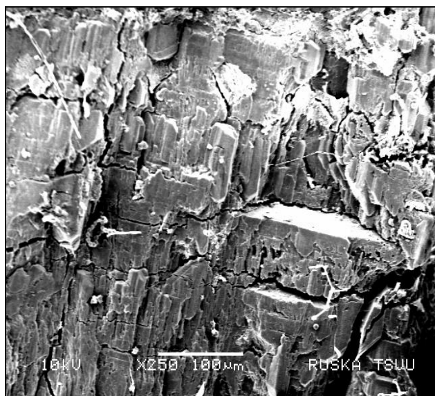
Fig.5: Scanning electron micrograph showing irregularly arranged rock like large magnesium ammonium phosphate crystals.
