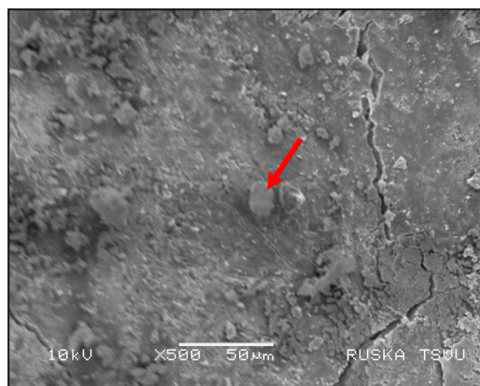
Fig.12: Scanning electron micrograph showing calcium oxalate monohydrate crystals.
