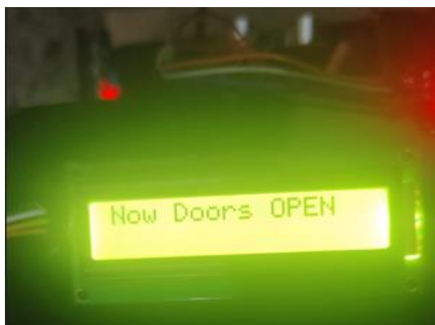
Fig.17: Showing LCD doors open Condition when train stopped in the station
