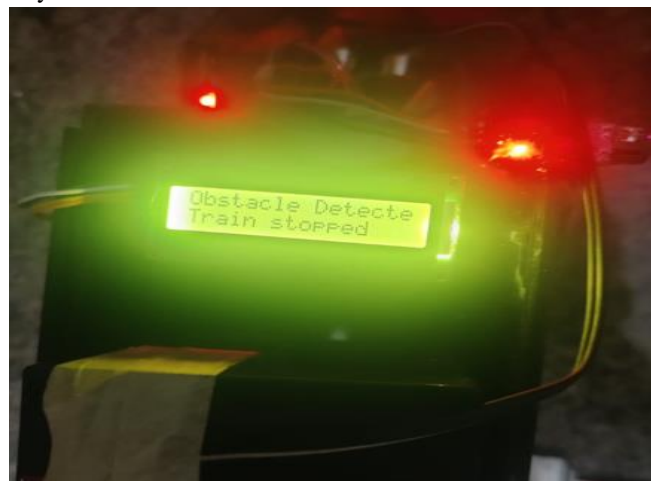
Fig.19: Showing LCD that train stopped when obstacle detected on the track
