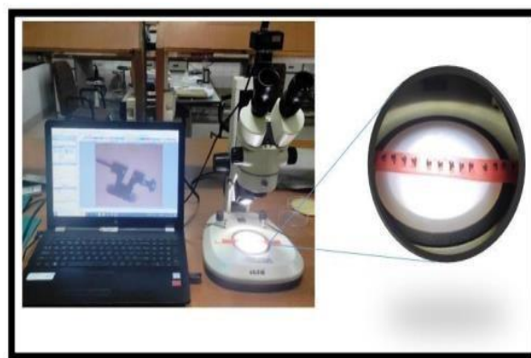
Fig. 3 Stereomicroscope, measuring software & brackets mounted on stereomicroscope slide
