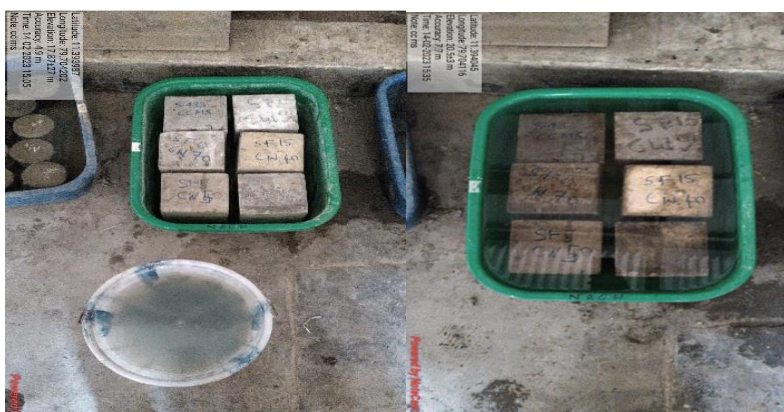
Fig.4 Specimens immersed in NaOH solution
