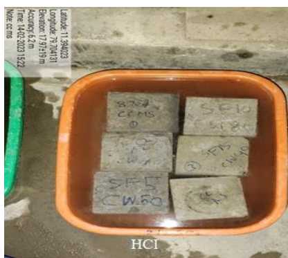
Fig.3 Specimens immersed in HCl acid
