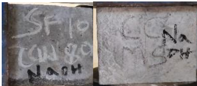
Fig.13 After 30 days of immersion in NaOH solution the visual appearances of the CCMS and CW80SF10 specimen
