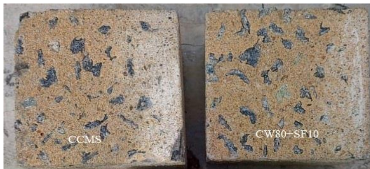
Fig.9 After 30 days of immersion in HCl solution the visual appearances of the CCMS and CW80+SF10specimens
