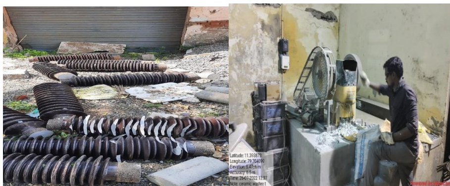
Fig.1 Process making of ceramic insulator waste as an aggregate
