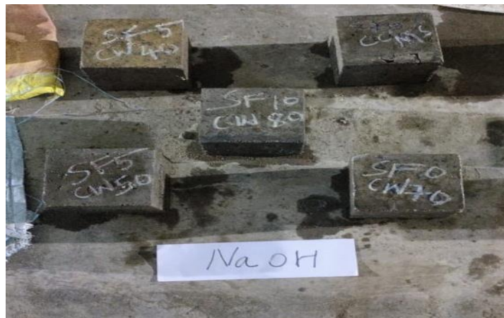
Fig.12 After 30 days of immersion in NaOH solution CCMS, CW70SF0, CW50SF5, CW80SF10 and CW40SF15 specimens
