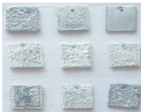
Figure 2: cross sections of coated mild steel samples
