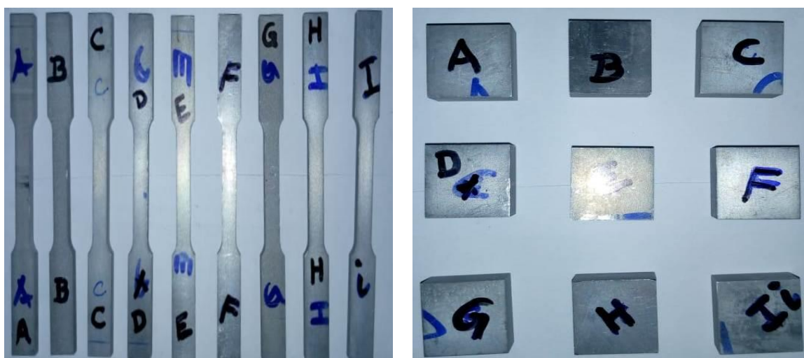
Fig 3. AMMC test samples as per ASTM standards
