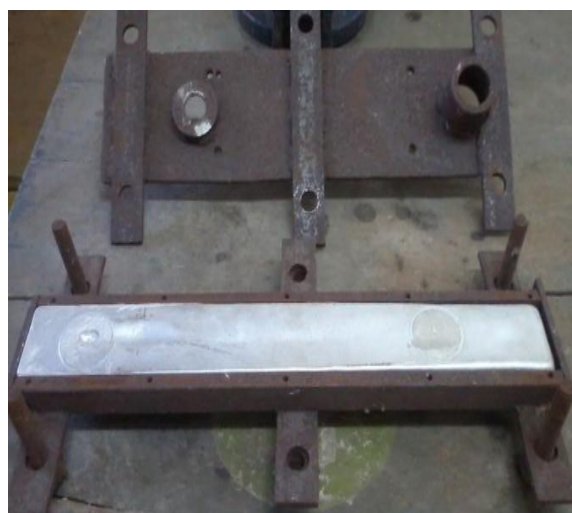
Fig 2. AMMC Sample with Die
