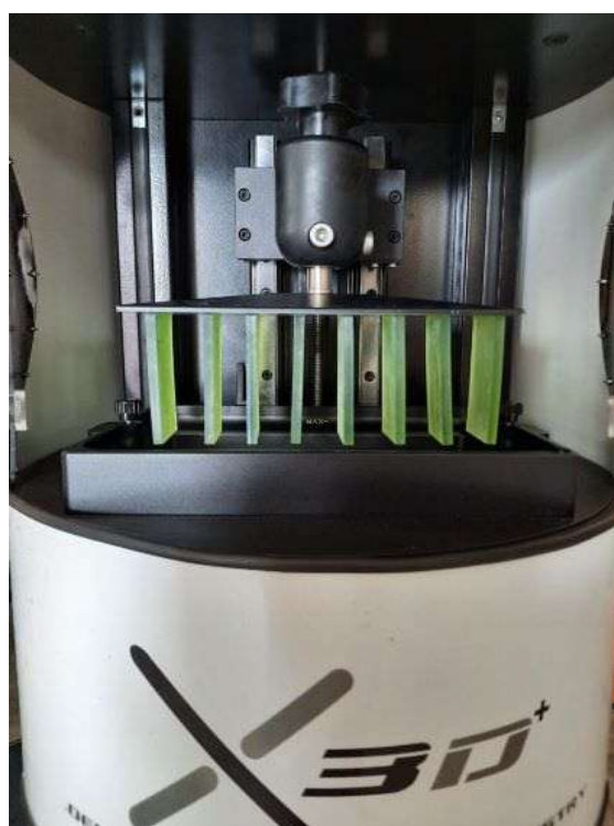
Figure 2. 3D Printing of Samples for Evaluating Surface Roughness and Flexural Strength
