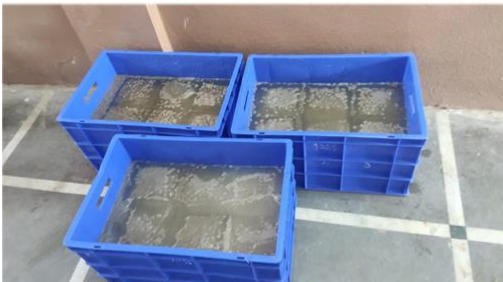
Fig.10: Immersion of cubes in 5% HCL AND 10 % HCL
