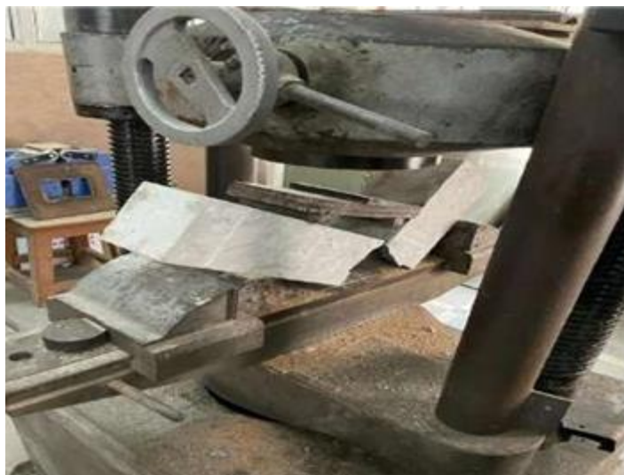
Fig .8: Flexural strength test
