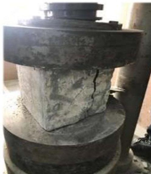
Fig. 2: Compressive Strength of Cube Specimens Table. 1: Compressive strength for 7 days
