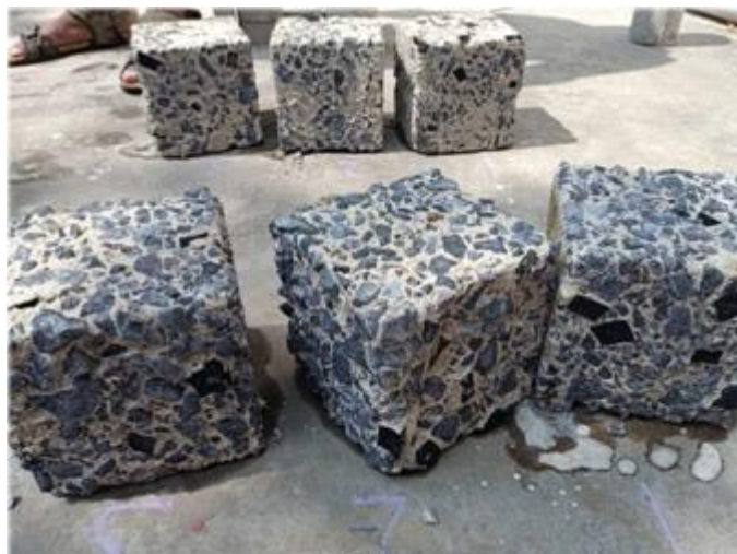
Fig. 11: 5% Hcl And 10 % Hcl Subjected Specimens
