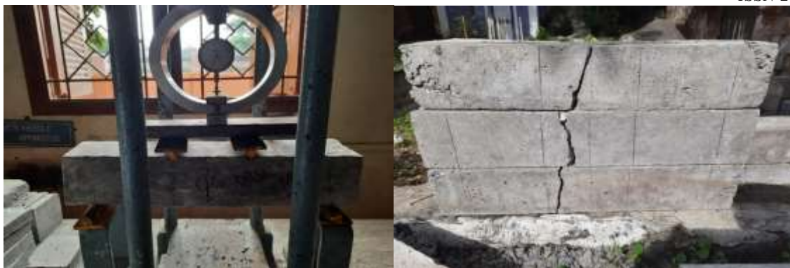
Fig.8 flexural strength testing and failure specimens
