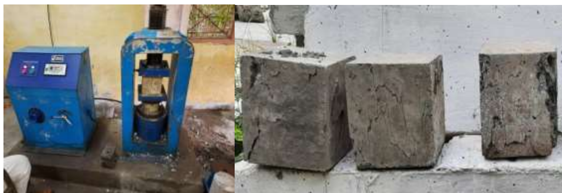
Fig.6 Testing and Failure modes of specimens
