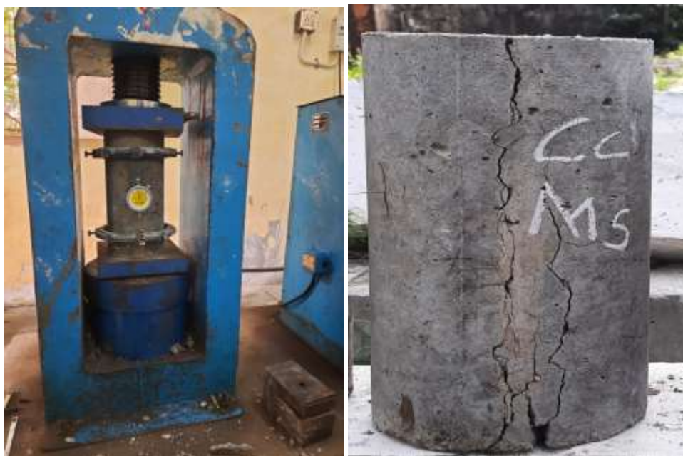
Fig.11 Modulus of elasticity testing and failure specimens
