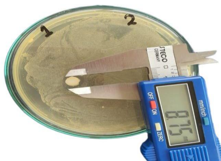
Figure 7: Measurement of inhibition zone around S-PRG resin composite (Group I)
