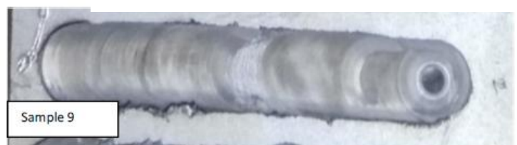
Fig 5: Specimen processed with threaded tool
