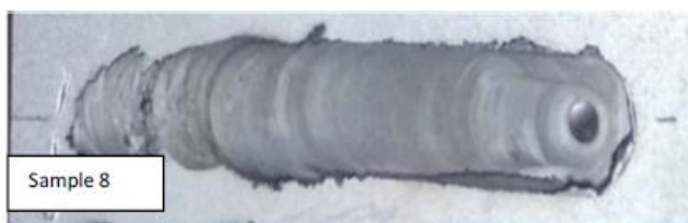
Fig 4: Specimens processed with conical tool
