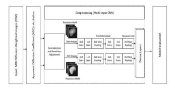
Fig. 2. Schematic diagram of our proposed CAD system that shows the design and the layers of the multi-input CNN deep-learning framework.
